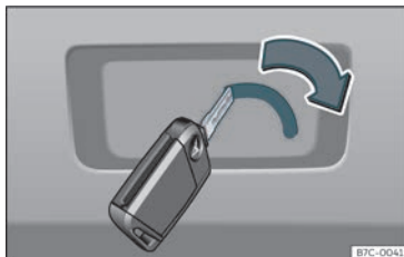
Fig. 82 Detail of the luggage compartment: emergency unlocking
