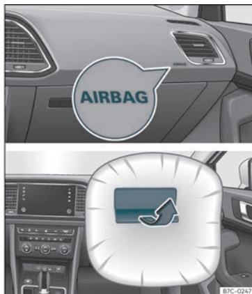
Fig. 13 Front passenger airbag located in dash panel.
