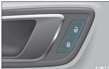
Fig. 70 Driver's door: central locking switch.
