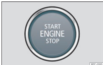
Fig. 197 In the lower part of the centre console: start button.
