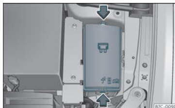
Fig. 45 In the engine compartment: fuse box cover.
