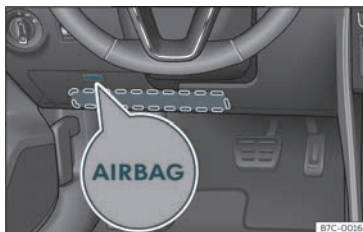
Fig. 16 On the driver side: location of the knee airbag
