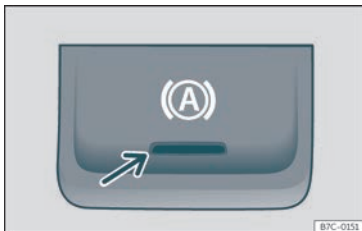
Fig. 231 In the lower part of the centre console: Auto Hold function button.
