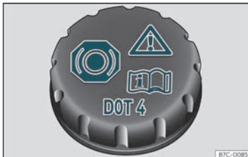
Fig. 261 Engine compartment: brake fluid reservoir cap.
