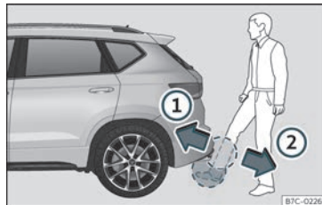
Fig. 80 Rear lid with sensor-controlled opening (Easy Open).
