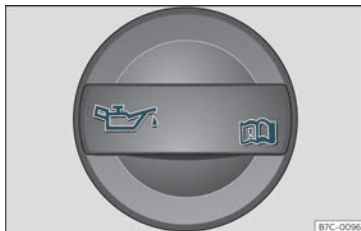
Fig. 258 In the engine compartment: Engine oil filler cap.
