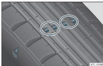
Fig. 264 Tyre profile: tread wear indicators.
