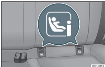
Fig. 24 Rear seat: ISOFIX/i-Size securing rings.
