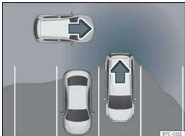
Fig. 229 Schematic representation of the rear cross traffic alert assistant: zone monitored around the vehicle while leaving a parking space.
