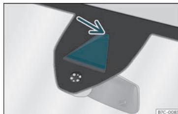
Fig. 222 On the windscreen: field of vision of the Lane Assist system.
