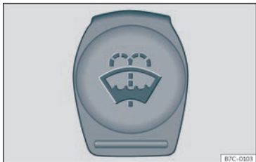
Fig. 262 In the engine compartment: window washer tank cap.
