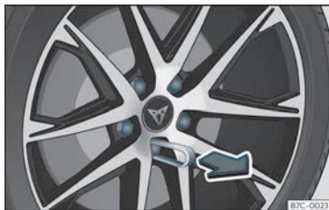
Fig. 30 Wheel: wheel nuts with caps.
