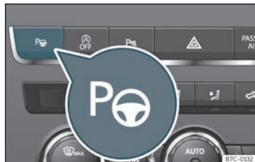
Fig. 232 In the upper part of the centre console: button to switch on the Park Assist system.
