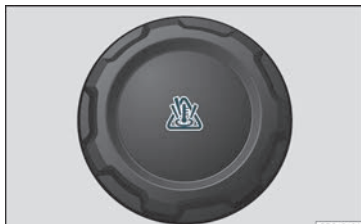
Fig. 260 Engine compartment: coolant expansion tank cap.
