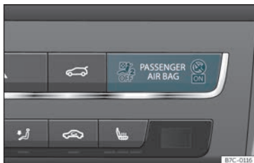
Fig. 15 Dash panel: control lamp for the deactivation of the front passenger front airbag.
