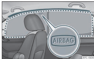
Fig. 20 Location of head-protection airbags.
