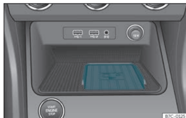
Fig. 196 In the centre console: pad for the mobile phone connection.
