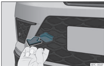
Fig. 39 On the right side of the front bumper: remove the cover.
