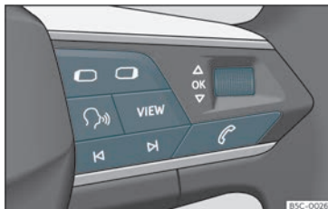
Fig. 62 Right side of the multifunction steering wheel: buttons to the menus and information displays on the instrument panel.
