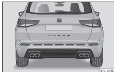
Fig. 151 Rear view of the vehicle: radar sensor zones.
