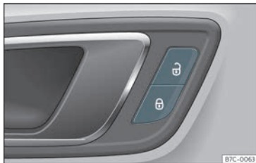
Fig. 75 Driver's door: central locking switch.
