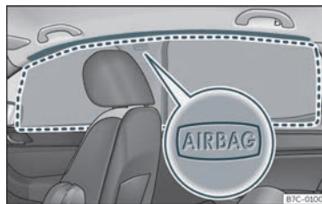
Fig. 21 Location of head-protection airbags.
