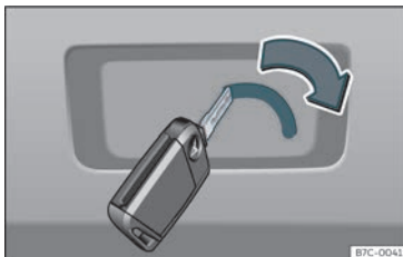
Fig. 87 Detail of the luggage compartment: emergency unlocking
