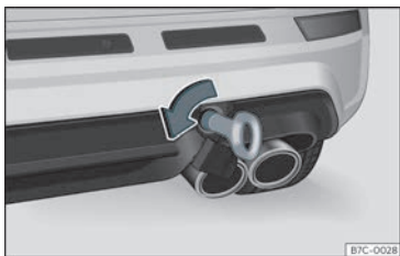
Fig. 44 On the right side of the rear bumper: towline anchorage in position.
