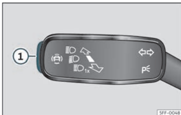
Fig. 63 On the turn signal and main beam lever: button for driver assistance systems (depending on versions).
