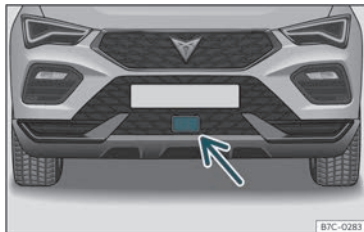
Fig. 148 On the front bumper: radar sensors.
