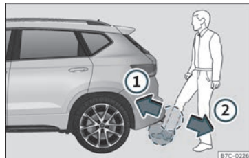
Fig. 85 Rear lid with sensor-controlled opening (Easy Open).
