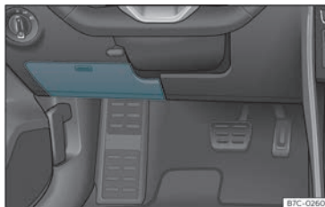
Fig. 45 Left hand drive vehicles: fuse box cover under the driver's side dashboard
