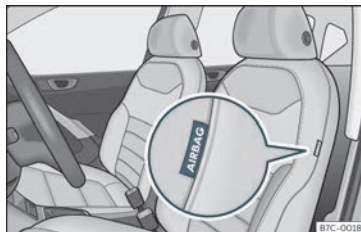
Fig. 19 Side airbag in driver's seat.
