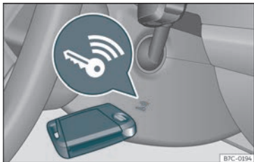
Fig. 140 On the right of the steering column: emergency start.
