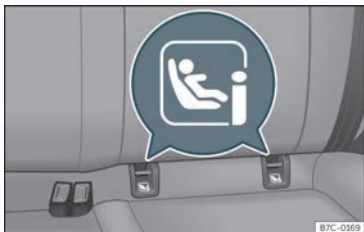
Fig. 25 Rear seat: ISOFIX/i-Size securing rings.
