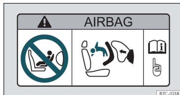
Fig. 23 Airbag sticker: on the passenger's sun visor
