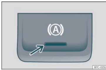
Fig. 176 In the lower part of the centre console: Auto Hold function button.
