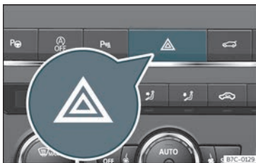
Fig. 95 Dash panel: hazard warning lights switch
