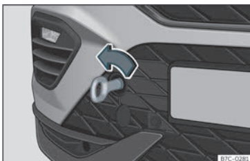
Fig. 42 On the right side of the front bumper: towline anchorage in position.
