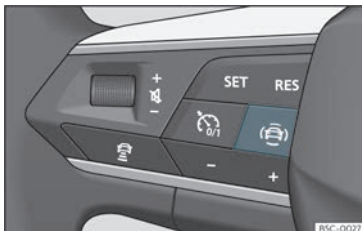
Fig. 64 Left side of the multifunction steering wheel: button for driver assistance systems (depending on versions).
