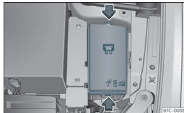
Fig. 47 In the engine compartment: fuse box cover.
