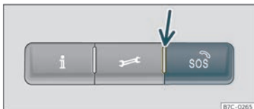
Fig. 29 On the roof console: voice service controls
