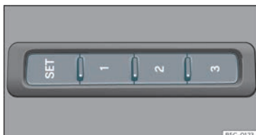
Fig. 106 On the outer side of the driver's seat: memory buttons.
