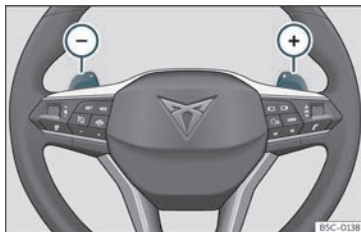
Fig. 144 Steering wheel: automatic transmission levers
