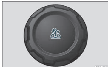
Fig. 205 Engine compartment: coolant expansion tank cap.
