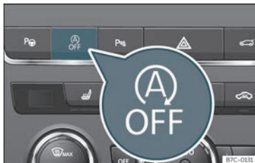
Fig. 141 Centre console: Start-stop system button.
