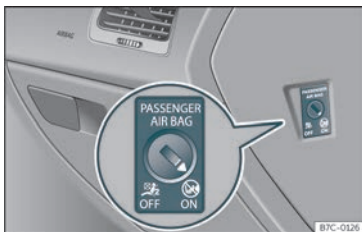
Fig. 15 Switch for activating and deactivating the front passenger airbag.
