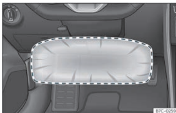
Fig. 18 On the driver side: airbag action radius for the knees.
