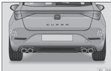
Fig. 162 Rear view of the vehicle: radar sensor zones.
