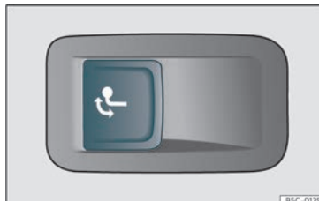
Fig. 198 On the left side of the luggage compartment: button for unlocking the tow hook.
