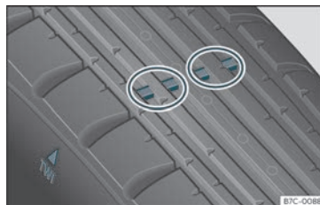
Fig. 224 Tyre profile: tread wear indicators.
