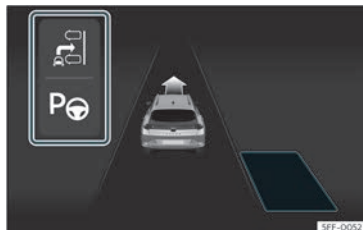
Fig. 189 On the instrument panel display: view of the parking assist system with reduced view.
