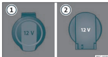
Fig. 140 12 volt power socket: ① inside the front armrest, ② in the luggage compartment.
