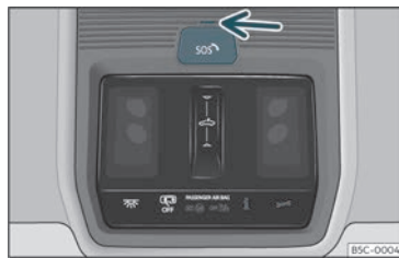
Fig. 36 On the roof console: voice service controls
