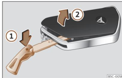
**Fig. 58** Vehicle key: opening the battery compartment cover.
