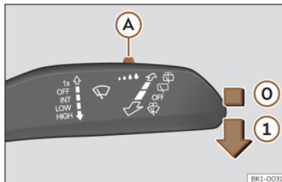
Fig. 86 Wiper lever: adjust the rain sensor
