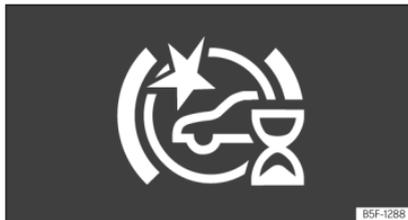
**Fig. 108** On the instrument panel display: initial system self-calibration indication.
