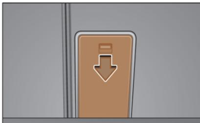
**Fig. 142** In the luggage compartment: opening the trapdoor.
