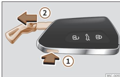
**Fig. 57** Vehicle key: remove the key blade.
