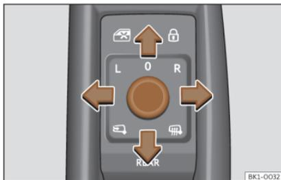
**Fig. 88** Detail of the driver's door: control for the exterior mirror.
