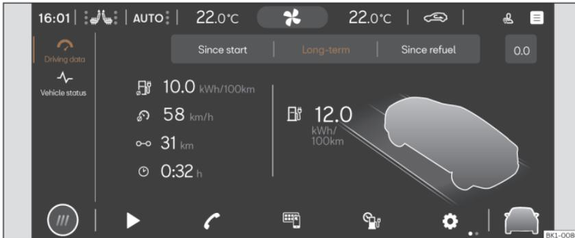
**Fig. 11** Schematic representation: Vehicle information and status
