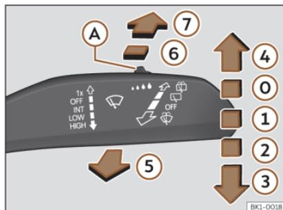
**Fig. 85** Operating the windscreen wiper and rear wiper.
