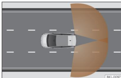
**Fig. 99** Sensor detection zones
