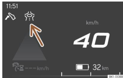
Fig. 8 Eco-efficient driving assistance indication (schematic representation).
