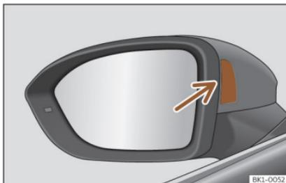
**Fig. 111** Control lamp of the lane departure warning.
