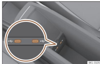
**Fig. 127** Inside the front centre armrest: USB port.
