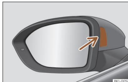
Fig. 117 In the mirror: warning lamp
