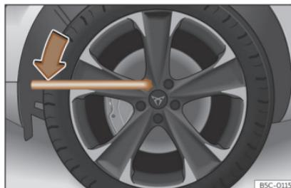
**Fig. 167** Wheel change: loosen the wheel nuts.
