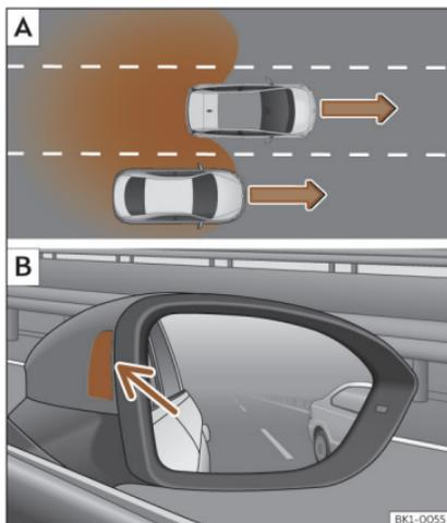
**Fig. 114** Schematic representation: **A** Situation of an overtaking in the centre lane and then moving into the right-hand lane. **B** Indication of the lane departure warning in the control lamp on the right side.
