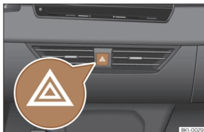
Fig. 40 Dash panel: hazard warning lights switch
