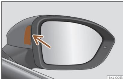
**Fig. 112** Control lamp of the lane departure warning.
