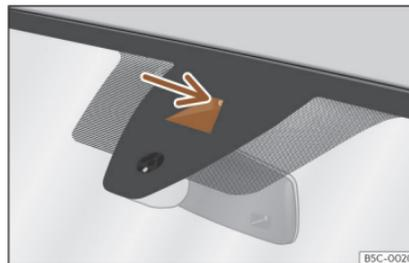
**Fig. 97** On the windshield: field of vision of the Lane Assist system.
