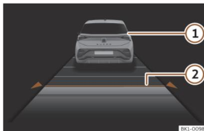
**Fig. 102** On the instrument panel display: ACC active.
