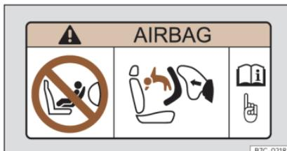
**Fig. 33** Airbag sticker: on the passenger's sun visor
