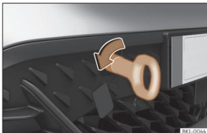
**Fig. 150** Right side of the front bumper: towline anchorage in position.
