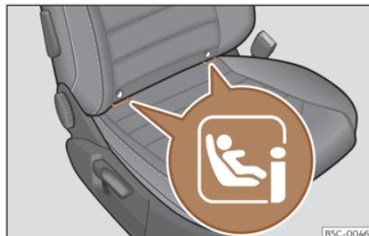
**Fig. 36** Front passenger seat: i-Size retaining rings.
