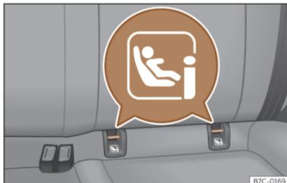
**Fig. 35** Rear seat: ISOFIX or i-Size securing rings.
