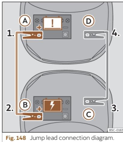
**Fig. 148** Jump lead connection diagram.
