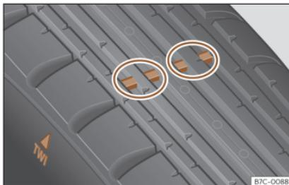
Fig. 162 Tyre profile: tread wear indicators.
