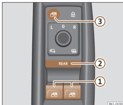
**Fig. 69** Detail of the driver's door: window controls.
