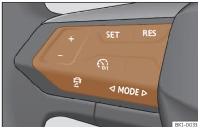
Fig. 70 Controls on the steering wheel.
