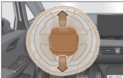
**Fig. 23** Driver airbag located in steering wheel.
