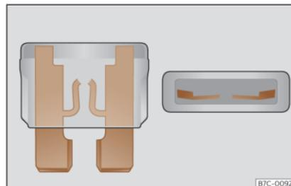
**Fig. 154** Image of a blown fuse.
