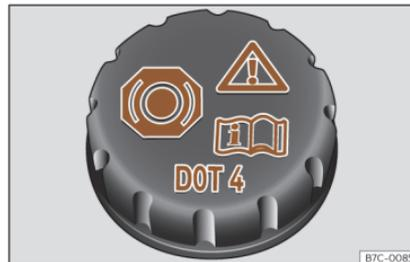
**Fig. 159** Front compartment: brake fluid reservoir cap.
