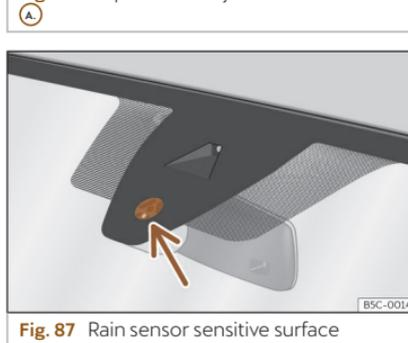
Fig. 87 Rain sensor sensitive surface
