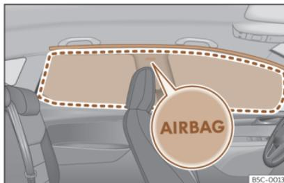
**Fig. 31** Location of head-protection airbags.
