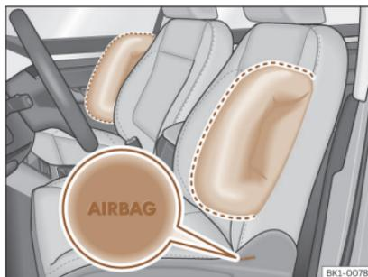
**Fig. 29** Driver's seat and passenger seat side airbags.
