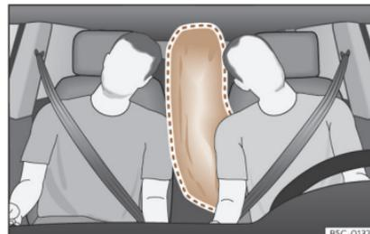
**Fig. 28** Fully inflated central airbag (deployment zone).
