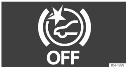
**Fig. 109** On the instrument panel display: Front Assist deactivated indication.
