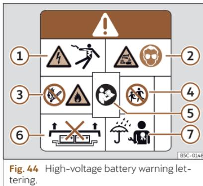
Fig. 44 High-voltage battery warning lettering.
