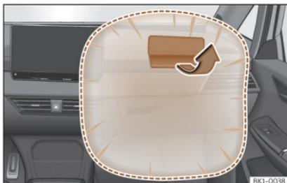
**Fig. 24** Front passenger airbag located in dash panel.
