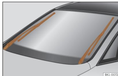
Fig. 144 Wipers in service position.
