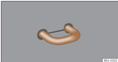
**Fig. 139** In the luggage compartment: fastening rings.
