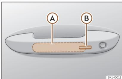
Fig. 61 Door handle: sensor surfaces
