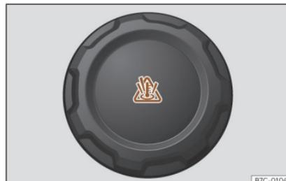
**Fig. 158** Front compartment: coolant expansion tank cap.
