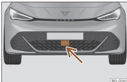
**Fig. 95** On the front bumper: radar sensors.
