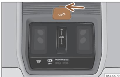
**Fig. 41** On the roof console: voice service controls
