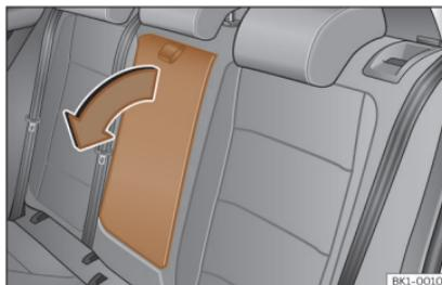
**Fig. 79** Folding rear centre armrest (schematic view).
