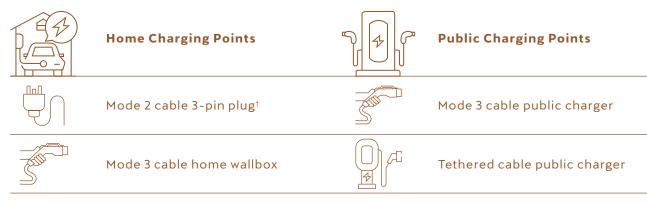
Home charging points tend to be AC (Alternating Current) which can charge your Born from 0-100% in under 7 hours.
