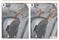
**Fig. 39** Rear seats: adjustment and assembly according to the Top Tether belt.
