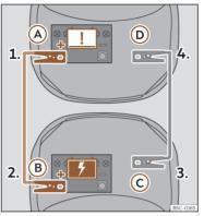
Fig. 166 Jump lead connection diagram.
