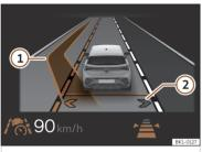
**Fig. 120** On the instrument cluster screen: lane change assist display (schematic representation).
