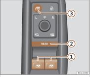
**Fig. 75** Detail of the driver door: controls for the windows.
