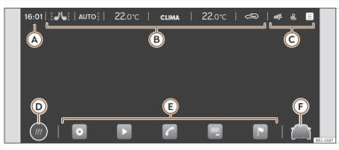
**Fig. 9** Schematic diagram: Overview of the possible function buttons on the screen.
