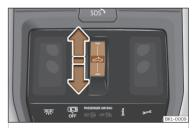
**Fig. 96** On the interior roof lining: function button to operate the sun blind.
