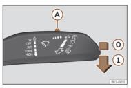
Fig. 92 Windscreen wipers lever: adjust the rain sensor (A).
