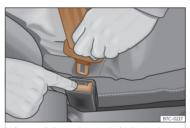
Fig. 21 Release the seat belt's latch plate.
