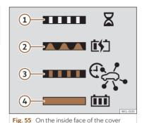
of the battery charging socket: sticker with information on the charging process display.
