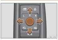
**Fig. 94** Detail of the driver door: control for the exterior mirror.
