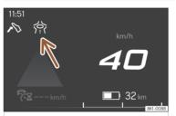
Fig. 8 Eco-efficient driving assistance indication (schematic representation).
