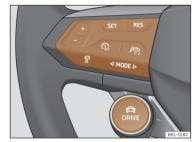
Fig. 76 Controls on the steering wheel.
