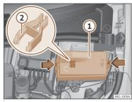
**Fig. 171** In the front compartment: fuse box cover.
