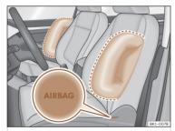
**Fig. 30** Driver's seat and passenger seat side airbags.
