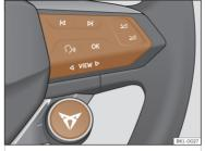
Fig. 77 Controls on the steering wheel.
