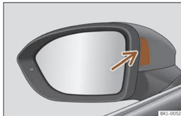
Fig. 134 Control lamp of the lane departure warning.
