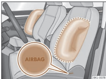
Fig. 32 Driver's seat and passenger seat side airbags.
