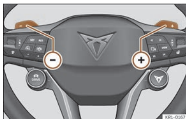
Fig. 107 Multi-function steering wheel: energy recuperation levers.
