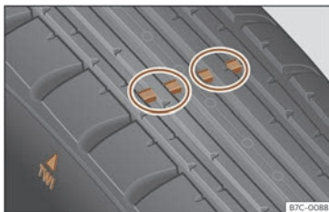
Fig. 206 Tyre profile: tread wear indicators.
