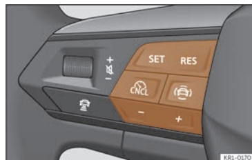
Fig. 119 On the multifunction steering wheel: buttons to control the speed limiter.
