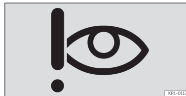
Fig. 6 On the instrument cluster display: Attention monitor symbol.
