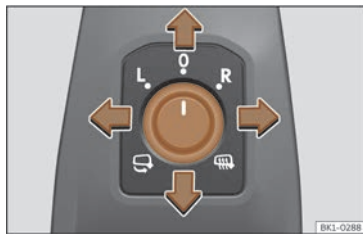
Fig. 101 Driver's door detail: exterior mirror control.
