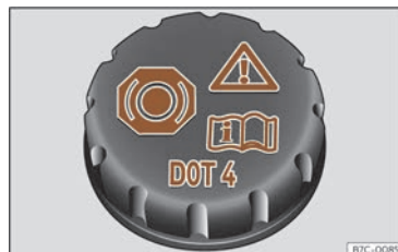
Fig. 203 Front compartment: brake fluid reservoir cap.
