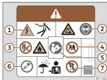
Fig. 53 High-voltage battery warning lettering.
