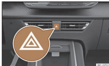
Fig. 47 Dashboard: hazard warning lights button.
