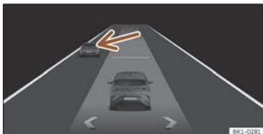
Fig. 123 On the instrument cluster display: ACC active, vehicle detected on the left.
