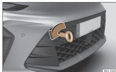
Fig. 194 Right side of the front bumper: towing eye screwed in.
