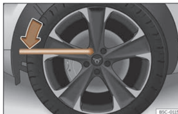
Fig. 211 Tyre change: loosen the wheel nuts.
