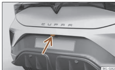
Fig. 117 On the rear bumper: location of the rear assist camera.
