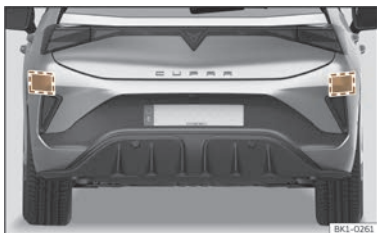
Fig. 115 Rear view of the vehicle: radar sensor areas.
