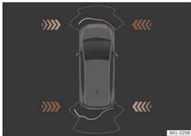
Fig. 128 In the infotainment system: junction assist display.
