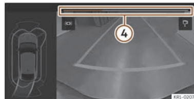
Fig. 145 On the infotainment system display: progress bar
