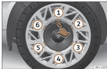
Fig. 208 Changing the wheel: removing the central trim.
