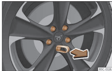
Fig. 209 Wheel: wheel nuts with caps.
