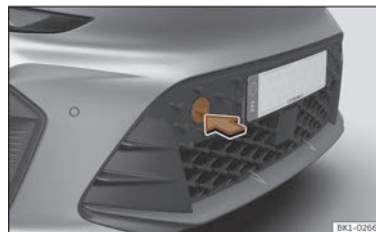
Fig. 193 Front bumper on right: remove the lid.
