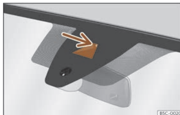
Fig. 114 On the windscreen: field of vision of the Lane Assist system camera.
