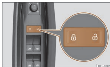
Fig. 75 On the driver's door: central locking button.
