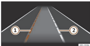
Fig. 129 On the instrument cluster display: indications of the lane assist system.
