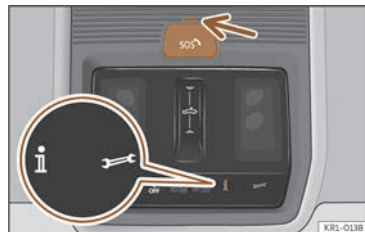
Fig. 48 On the roof console: controls for voice services.
