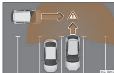
Fig. 151 Park assist diagram: detected area around the vehicle that is driving off.
