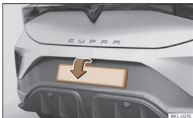
Fig. 177 Rear of vehicle: number plate bracket.
