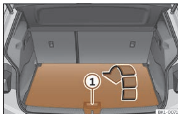
Fig. 171 In the luggage compartment: open the second luggage compartment floor.
