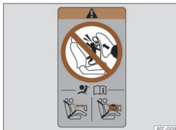
Fig. 37 Airbag sticker: on the rear frame of the passenger side door.
