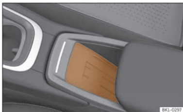
Fig. 164 On the centre console: pad for the mobile phone connection.
