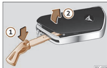
Fig. 70 Vehicle key: open the battery compartment cover.
