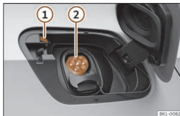
Fig. 57 Behind the battery charging cover on the rear right-hand side: Charging socket
