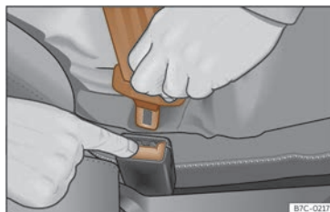
Fig. 23 Release the seat belt's latch plate.
