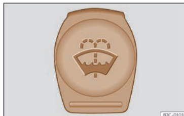
Fig. 204 In the front compartment: blue cap of the windscreen washer reservoir.
