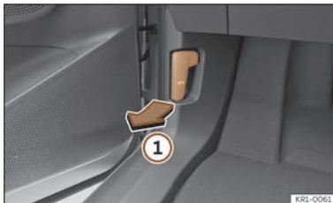
Fig. 199 Release lever in the driver's footwell area.
