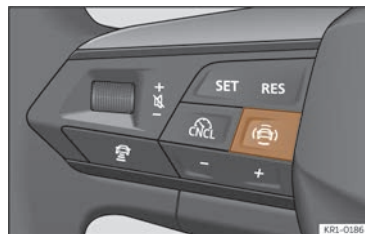
Fig. 111 Left side of the multifunction steering wheel: button for driver assistance systems (depending on the version).
