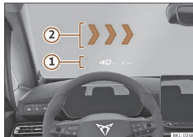
Fig. 4 In the driver's field of view: Proximity HUD ① and AR HUD ②.
