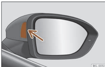
Fig. 135 Control lamp of the lane departure warning.
