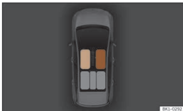
Fig. 19 Instrument cluster: seat belt status display.
