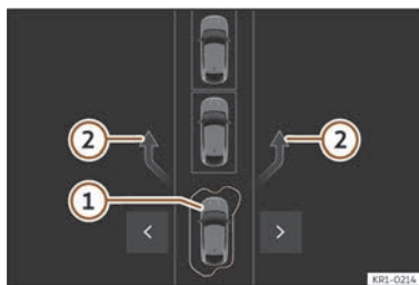
Fig. 147 On the infotainment system display: leaving a parallel parking space.
