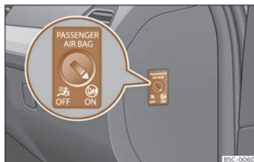
Fig. 28 Switch for activating and deactivating the front passenger airbag.
