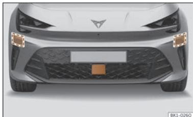
Fig. 112 On the front bumper: front and side radar sensors.
