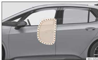
Fig. 33 Illustration of completely inflated side airbag on the left side of the vehicle.
