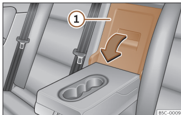
Fig. 183 On the rear seat backrest: opening the tailboard.
