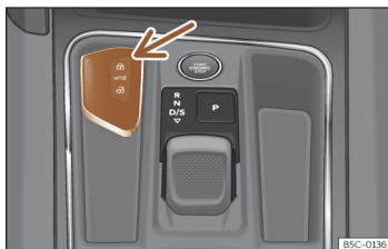
Fig. 64 Centre console: vehicle key housing.
