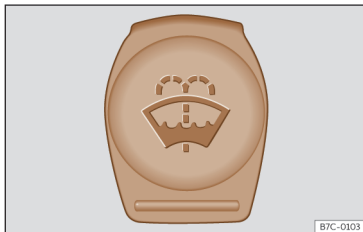
Fig. 212 In the front compartment: blue cap of the windscreen washer tank.
