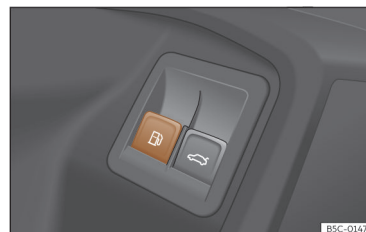
Fig. 192 Driver's door: tank cover release.
