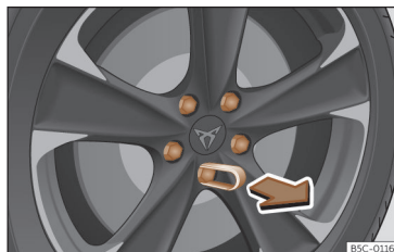
Fig. 224 Wheel: wheel bolts with caps.
