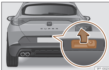
Fig. 75 Rear lid: opening from the outside.
