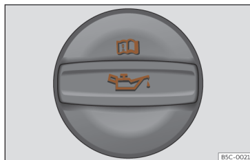
Fig. 216 Oil filler cap cover in the engine compartment.
