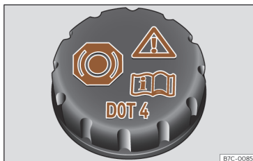
Fig. 211 Front compartment: brake fluid reservoir cap.
