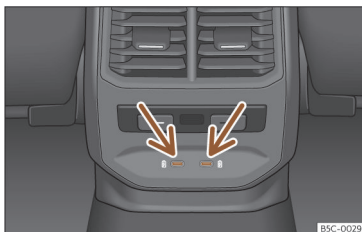
Fig. 166 Rear centre console: USB connectors with power socket function.
