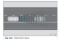
A radar sensor may be fitted to the front bumper of the vehicle>>> Fig. 140. The front radar detects any objects in its detection
