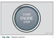
The engine can be started with a start button (Press & Drive). For this there must be a valid key inside the passenger compartment.
