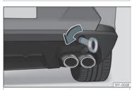
**Fig. 46** On the right side of the rear bumper: towline anchorage in position.
