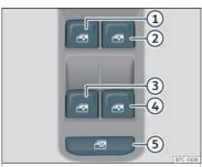
**Fig. 82** Detail of the driver's door: window controls.
