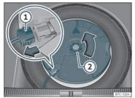
**Fig. 198** In the luggage compartment: remove the subwoofer.
