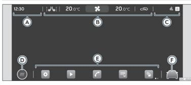
**Fig. 59** Schematic representation: Overview of the possible function buttons on the screen
