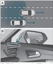
Fig. 163 Schematic representation: A Situation of an overtaking in the centre lane and then moving into the right-hand lane. In Indication of the lane departure warning in the control lamp on the right side.
