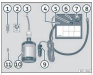
Fig. 34 Standard representation: anti-puncture kit contents.
