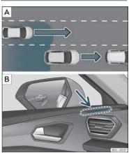
Fig. 162 Schematic representation: A Passing situation with traffic behind the vehicle. B Indication of the lane departure warning in the control lamp on the left side.
