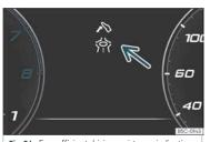
**Fig. 54** Eco-efficient driving assistance indication (schematic representation).
