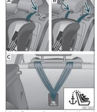
Fig. 29 Rear seats: adjustment and assembly according to the Top Tether belt.
