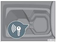
Fig. 135 In the centre console: emergency start.
