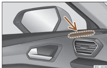
Fig. 157 Door: warning lamp
