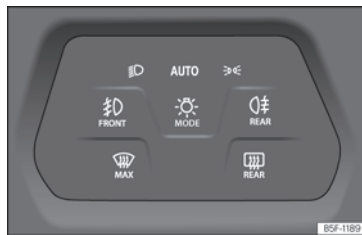
Fig. 99 Instrument panel: light panel.
